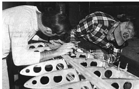
BUILDING THE WING - As Jim Gladney holds the rib steady, Charles Drew installs a fastener through the "drag strut" along the trailing edge of the wing. Fasteners projecting upward along the ribs in the foreground hold thin alignment strips in place.
